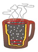
Stirring makes the fluid to rotate at uniform speed (left picture). Sugar is distributed uniformly in the cup.
